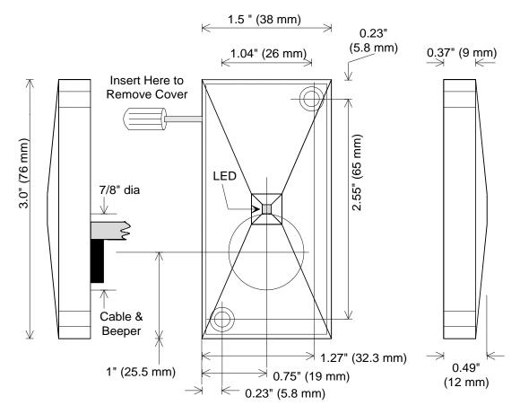
Figure 1 – P-300 Mounting Dimensions
