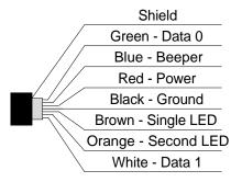
Figure 2 – Wiring Connections
